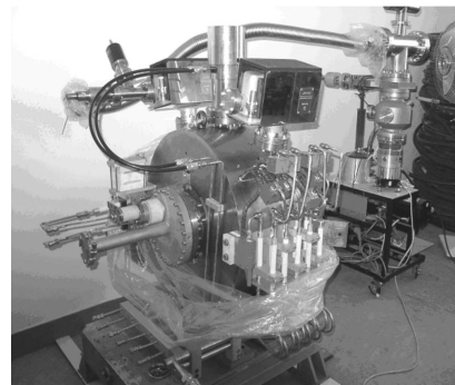
Fig. 2. Picture of the e^+ converter assembly.
