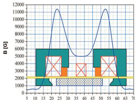
Fig. 1. The scheme of the magnetic structure and the axial magnetic field distribution.
