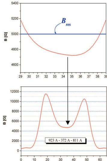
Fig. 3. Axial magnetic field distribution optimized for maximum yield of  $\text{Ar}^{8+}$ .
