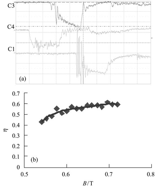
Fig. 5. (a) The typical waveform of the total current C3 and that of the beam current C1 (C4 is the waveform of the electron energy); (b) relationship between  $\eta$  (the ration of the beam current and the total current) and magnetic field  $B$ .
