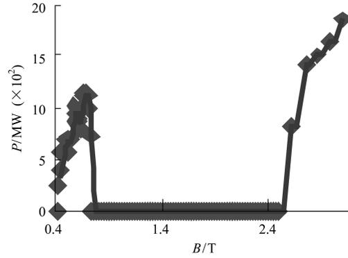
Fig. 8. The relationship between the output power and the guiding magnetic field.
