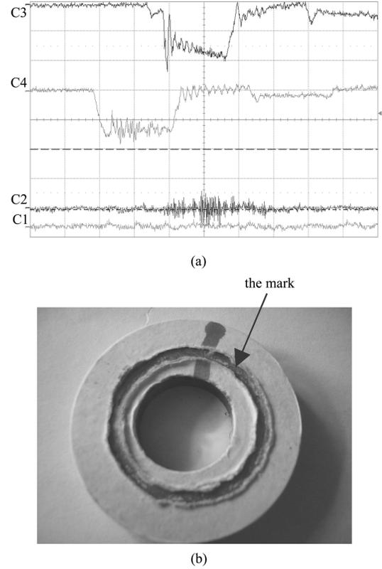
Fig. 4. (a) The waveform of the electron energy C4 and that of the beam current C3 (b) the mark of the electron beam.
