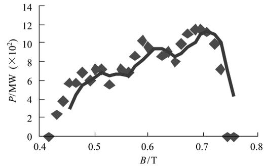
Fig. 9. The relationship between the output power and the guiding magnetic field when the magnetic field is small.
