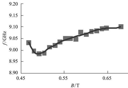
Fig. 11. The relation between the microwave frequency and the guiding magnetic field.
