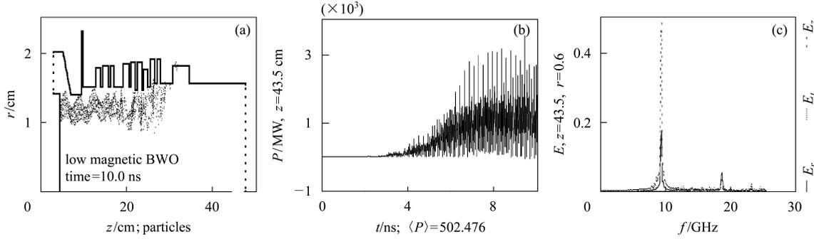
Fig. 1. (a) The model of BWO; (b) The output power vs time; (c) The frequency spectrum.
