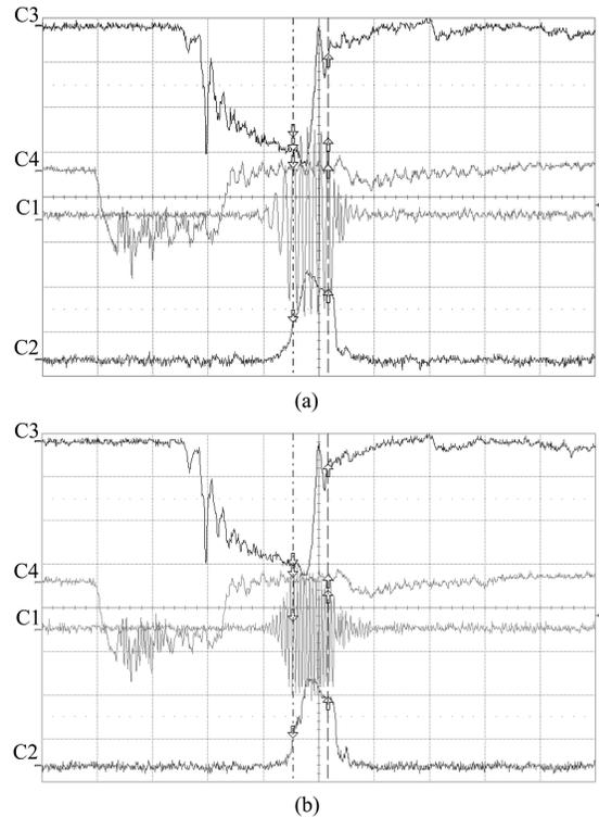
Fig. 2. The typical heterodyne signal (C3-IF signal, (a) when the fundamental is 9.5 GHz; (b) when the fundamental is 10 GHz).
