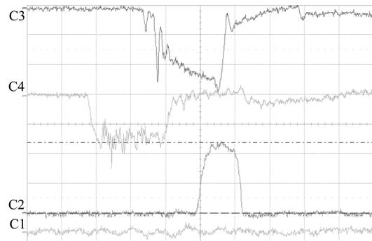
Fig. 10. The waveform (C4-of electron energy C3-of total current C2-of microwave detector signal).
