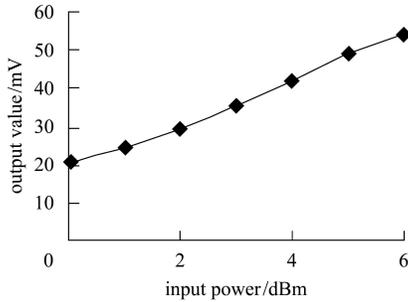
Fig. 3. The detecting curve of the detector.
