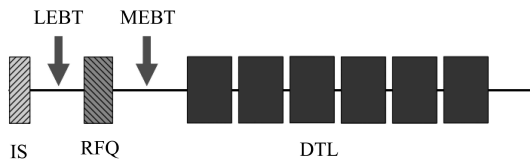
Fig. 2. Sketch map of the 35 MeV linac. IS: Ion Source; LEBT: Low Energy Beam Transport; MEBT: Medium Energy Beam Transport.
