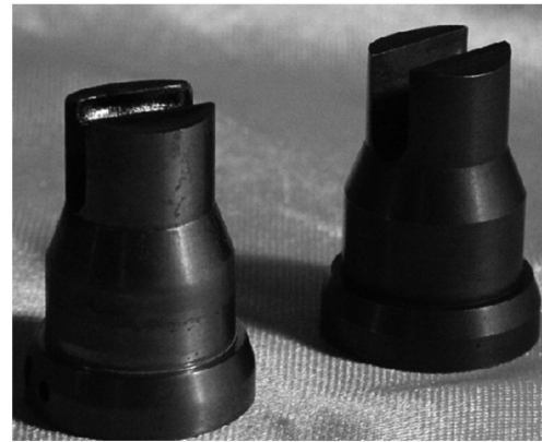
Fig. 6. (color online) Used cathode (left) and unused cathode (right). For the used cathode, the surface erosion is obvious on its surfaces.
