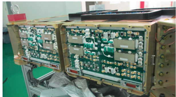
Fig. 5. (color online) Side view of the +X TRBs mounted on the STK framework.
