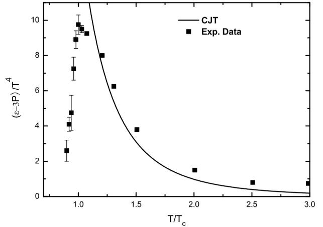
Fig. 2.  $(\epsilon - 3P)$  normalized by  $T^4$  as a function of  $T/T_c$  at  $\mu=0$ , with data points from Ref. [19]. The line represents the CJT results at  $\mathcal{B} = 255 \text{ MeV}/\text{fm}^3$ .
